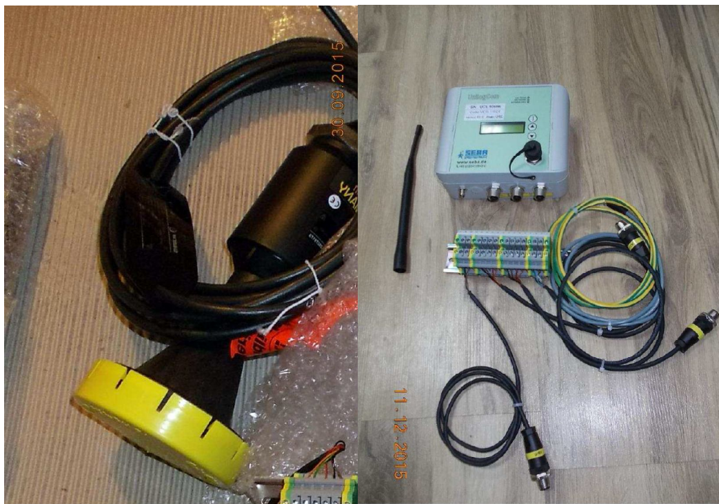
(Radar senzor tip SEBAPuls15, HS Kakanj n/B)
